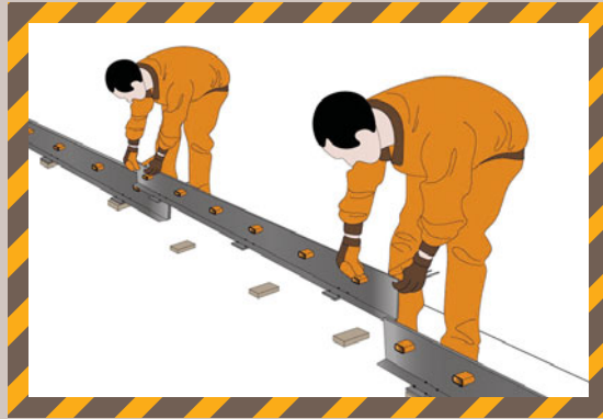
Positioning on the joint line.
